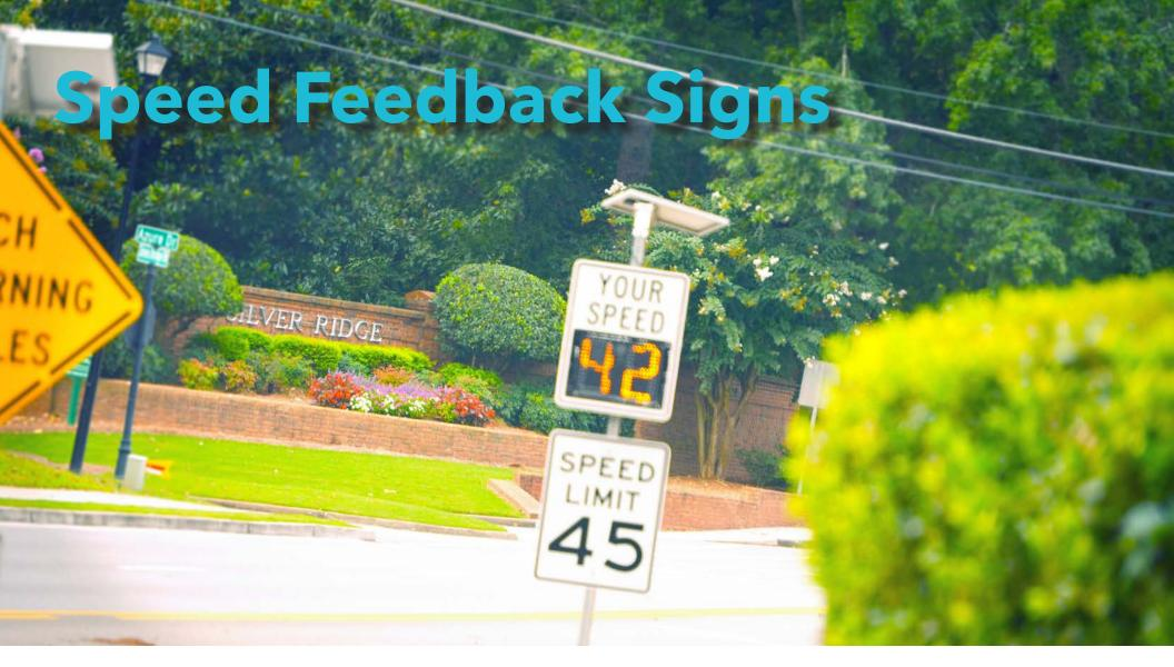
Speed feedback signs are permanently mounted signs that measure each approaching vehicle's speed and display it in view of the driver. The display can be set for flags when measured speed exceeds the posted limit. Speed feedback signs are typically mounted on or near speed limit signs.
