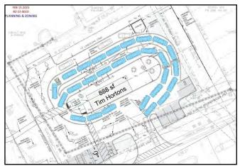
As a supplement to the trip generation report, a queuing analysis was conducted by Kimley-Horn and Associates on behalf of the Applicant, to observe and report on the traffic pattern on Abberley Lane and provide a comparative queuing analysis of a comparable use and similar private road with easement at the Starbucks on 4180 Old Milton Road. Both observations were conducted on a single weekday during the AM peak hour.
