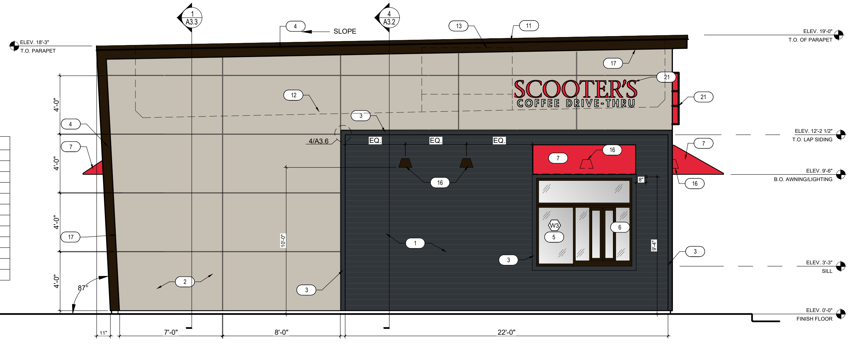
4 EXTERIOR ELEVATIONS SCALE: 1/4" = 1'-0"
